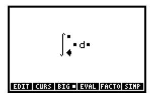
Enter values for all the "dots" by entering the desired values and then pressing the [RIGHT ARROW] button to move to the next location. A possible input could look like this.
