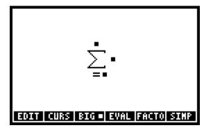
Enter values for all the "dots" by entering the desired values and then pressing the [RIGHT ARROW] button to move to the next location. A possible input could look like this.
