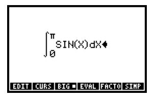
It should be noted that in the equation writer the calculator can integrate with respect to any variable, just make sure to put the desired variable in the differential. Once the integral is set up correctly, press [ENTER] to output the expression onto the stack.
