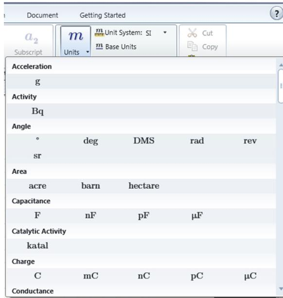
Mathcad displays units based on one of three “Unit Systems”: **SI**, **US Customary System (USCS)**, or **Centimeter-Gram-Second (CGS)**. The worksheet system is shown on the **Math** tab in the **Units** group.
